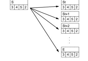
BSET(71) can be used to change timer/counter PV. (This cannot be done with MOV(21) or MVN(22).) BSET(71) can also be used to clear sections of a data area, i.e., the DM area, to prepare for executing other instructions.
